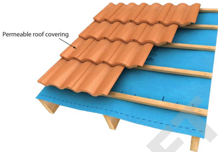
Figure 1: Cold Roof detail with permeable roof covering
