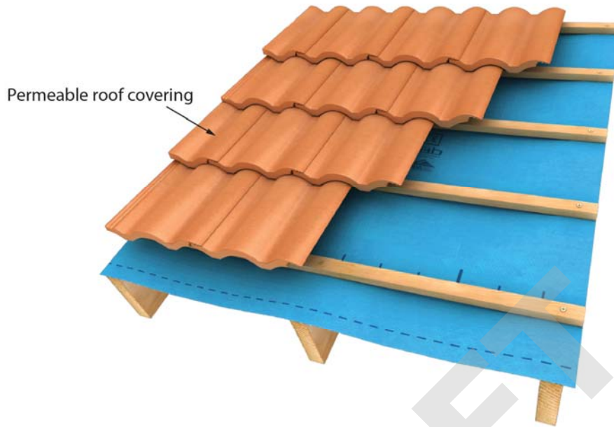
Figure 1: Cold Roof detail with permeable roof covering
