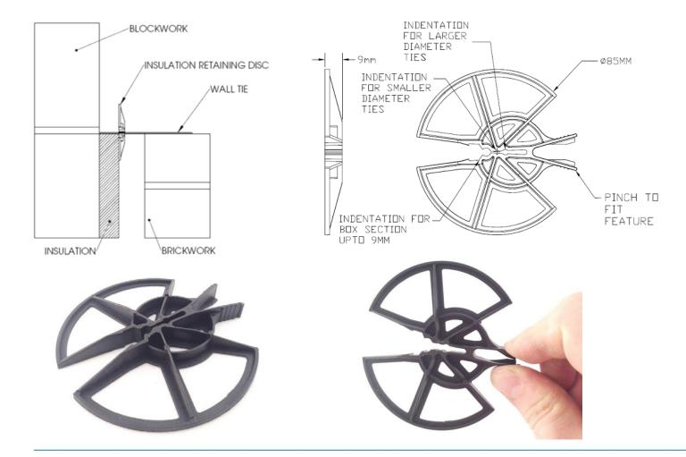
The KV9980 is an easy to use insulation retaining disc, designed to be used with fibre slab and rigid board insulation. With its unique "pinch to fit" design it reduces stresses put on the wall tie during installation which can often lead to bent or broken wall ties and also makes installation easier as the KV9980 can be installed with one hand.
