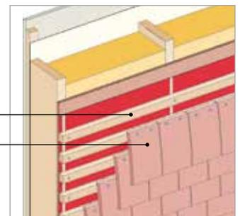
Note: Klobber recommend that 19mm deep counter battens are used on sites that are severely exposed.
