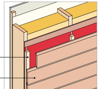
Treated timber battens gauged to suit tile size
