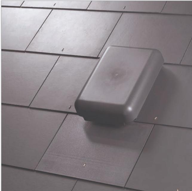
Large Slate Vent is a large capacity ventilating slate to suit 600mm x 300mm (24" x 12") and 500mm x 250mm (20" x 10") double lap slates, man-made or natural, for roofs with a pitch over 22.5°.
