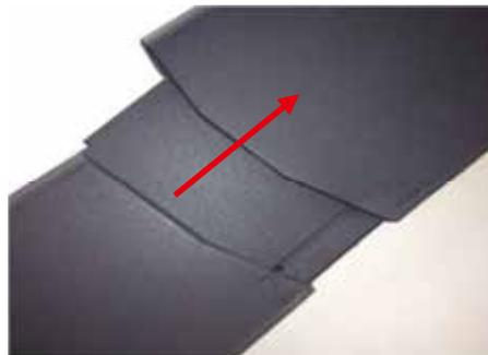
6. As each successive verge tile is laid, slide on a Uni-Click Dry Verge Unit up to the bottom of the tile, engaging with the Unit below, nail in position through the Batten End Clip into the batten.
