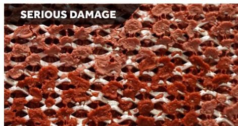
COMPETITOR B A two-layer product with serious damage, where the product has broken down.
