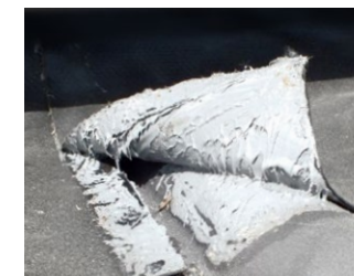
Competitor products using a full butyl connection instead of self-welding, can more easily fail, as seen here.
