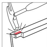
**Extra instructions for Thin-Line Tile Vent:** When used with a Quinn Lakeland Slate or Russell Galloway tile profiles, you may have to remove the side lock nib from the tile, as shown.
