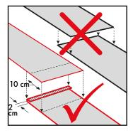
To join two pieces of EasyForm fold back 20mm minimum so butyl from the lower section meets the butyl from the upper section. This should form part of a 100mm overlap.
