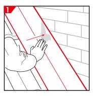
To form a single piece step and cover flashing for use on a profiled interlocking tile, select a piece of 450mm wide EasyForm of suitable length. This should be positioned to form a fold line allowing 150mm minimum vertical upstand and a minimum 150mm wide, or cover to a complete pan and roll horizontally.
