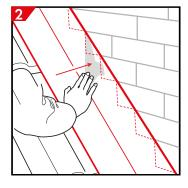
Next mark out and cut lines to form the steps from the vertical section as you would with lead ensuring a 65mm minimum vertical upstand is maintained before any cuts. Remember to allow 30mm for chasing into the brickwork
