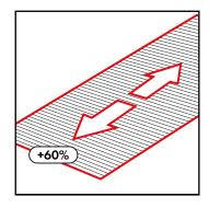
EasyForm can stretch up to 60% in the direction of the roll to enable dressing into the pan of the tile.
