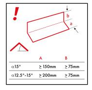
Ensure the correct overlap in relation to the roof pitch.
