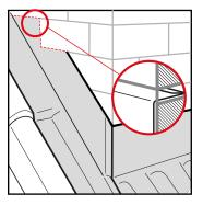
When dressing into a brickwork joint allow 30mm to ensure EasyForm is able to return. Complete with Klober Flashing Sealant (PACCSE). Secure with wedges and complete with Klober Flashing Sealant (PACCSE).
