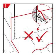
Position a length of 250mm or 300mm EasyForm on a clean, dry and dust free surface.
