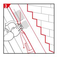
Place the EasyForm into position, gradually peel off the backing paper to the vertical section and press into place. The stepped detail should be completed by dressing the EasyForm into each brickwork joint. Finally, remove the backing paper from the lower section and carefully work onto the tile surface.
