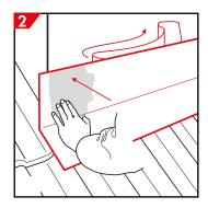
Remove the protective film from the upper section of EasyForm and carefully dress into the brickwork joint. This can be secured with wedges before finishing with Klober Flashing Sealant (PACCSE). Press the remainder of the vertical section against the brick wall.
