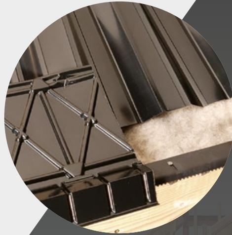
As well as providing the necessary ventilation openings from outside, we need to ensure that this ventilation air is able to reach the intended area. For a new build solution the Roll Out Rafter Tray (p35) works alongside the Over Fascia Vent (p39) to create a path for airflow into the roofspace, ensuring it is able to bypass any loft insulation that may otherwise block this route.
