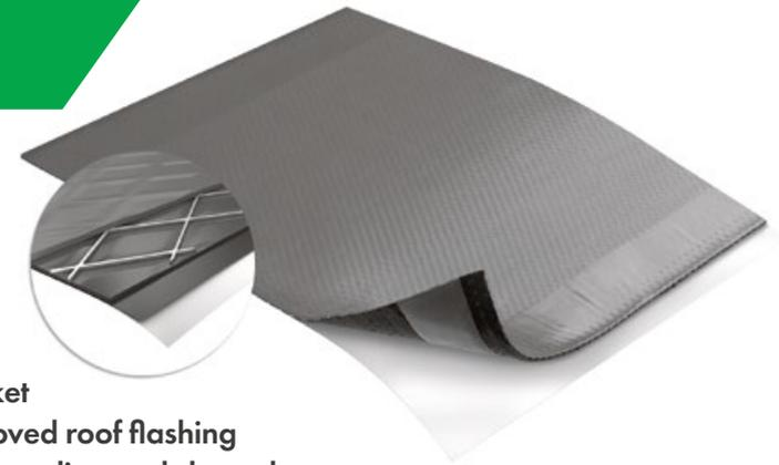
Wakaflex is a market leading, BBA approved roof flashing made from aluminium diamond shaped mesh embedded into UV resistant PIB (Polyisobutylene) with butyl strips to help prevent wind-uplift and release foil to protect the product prior to use.
